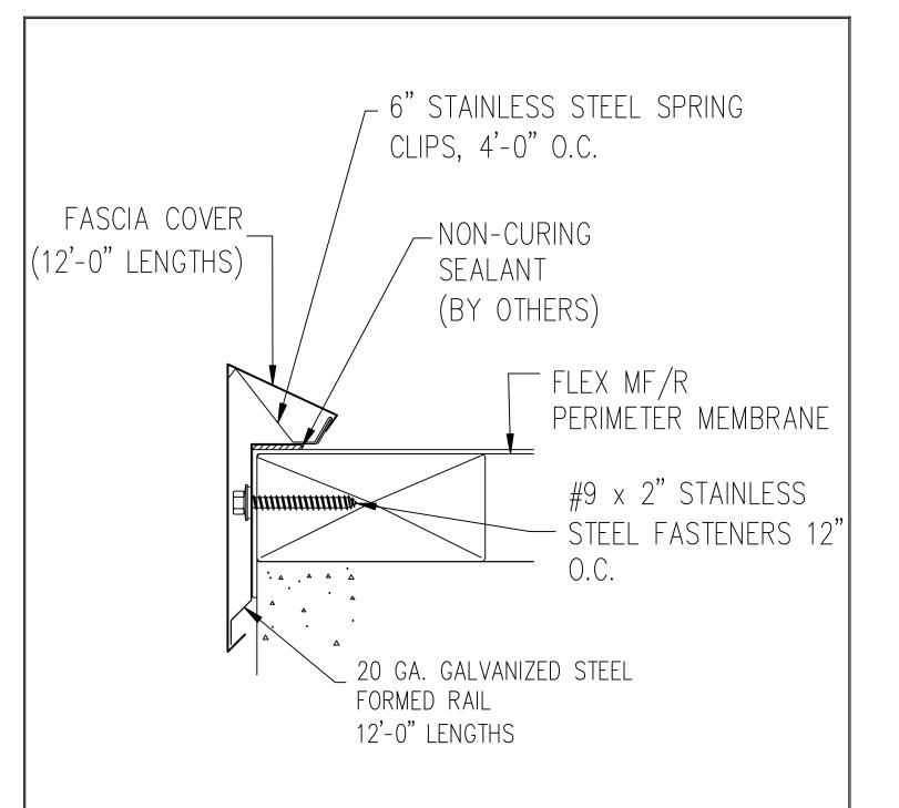
FLEX TPD: FLEX TPD CUT EDGE SEALANT IS REQUIRED ON ALL NON FACTORY CUT EDGES OF FLEX TPD
